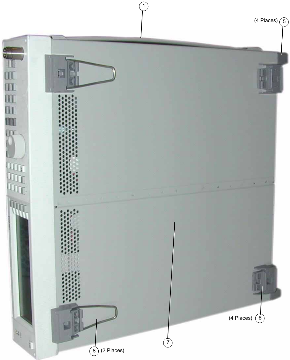
Figure 3-8 Outer Instrument Cover and Associated Parts
