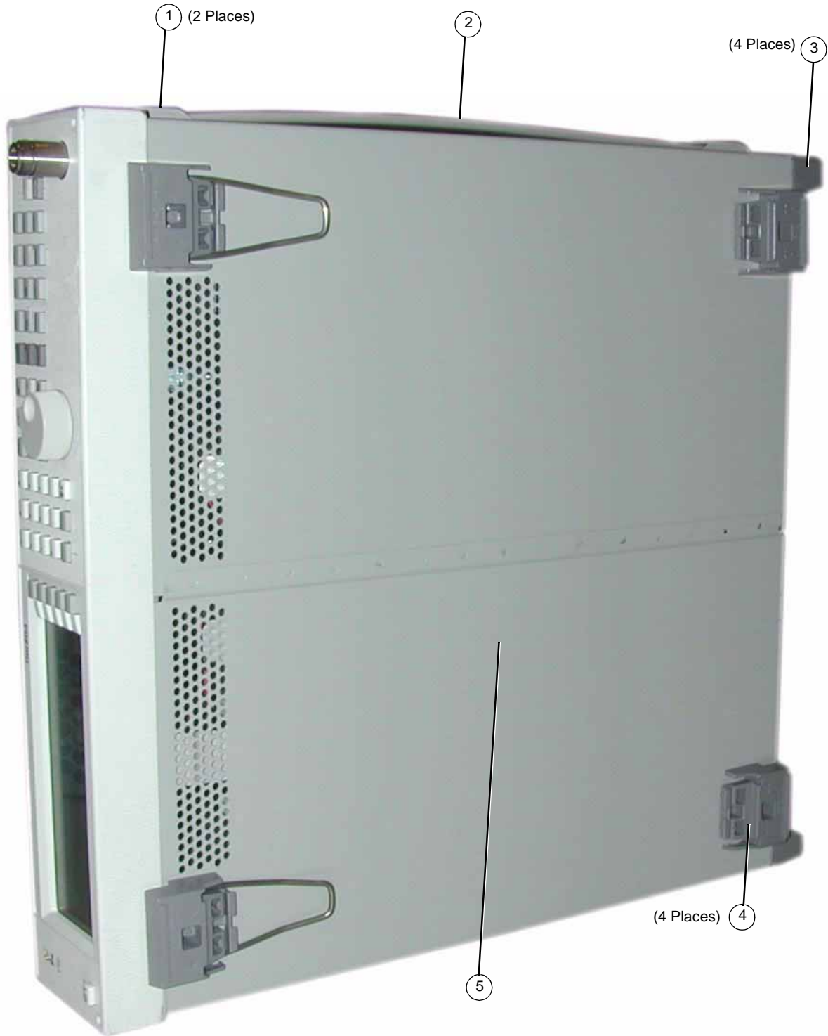
Figure 2-1 Outer Cover Removal
