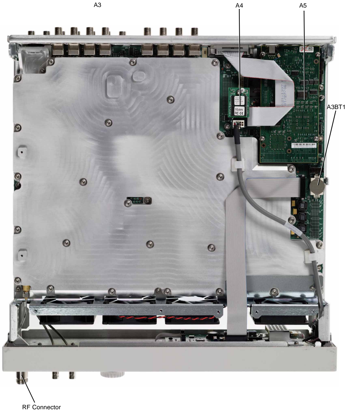
Figure 3-2 Assemblies from a Bottom View
